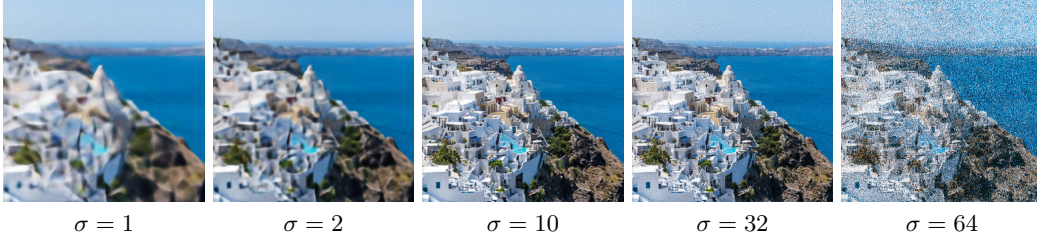
Figure 10: A visualization of the 2D image regression task with different Gaussian scales (corresponding to points along the curve shown in Figure 9). Low values of \sigma underfit, resulting in oversmoothed interpolation, and large values of \sigma overfit, resulting in noisy interpolation. We find that \sigma = 10 performs best for our Natural image dataset.
