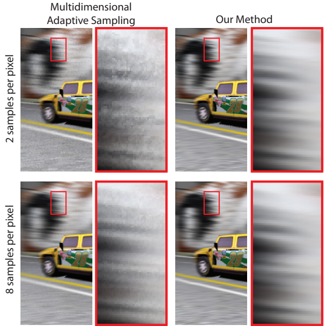
Figure 13: We show further results for our method and MDAS with 2 samples per pixel and 8 samples per pixel. For 2 samples per pixel our method does well for areas with uniform motion (in fact many areas use one sample per pixel and are in their final state), but does poorly for pixels where we detect a large difference between a_{\min} and a_{\max} . At 8 samples per pixel our method devotes all of the new samples to the difficult areas, and many places such as the shadows improve dramatically. MDAS by comparison starts out with fairly uniform noise, and then improves evenly over all areas of the image. The insets show that in areas with fairly uniform motion our method computes high-quality results at extremely low sample counts.
