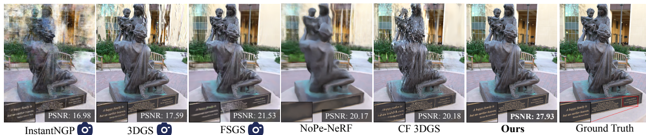
Figure 1: We introduce a sparse view synthesis method, which does not rely on off-the-shelf estimated camera poses. Given the “Family” scene in the Tanks & Temples dataset, we use 6 out of 200 frames as training views and others for testing. Compared with other pose-free methods, including COLMAP-Free 3DGS [Fu et al. 2023] (CF 3DGS) and NoPe-NeRF [Bian et al. 2023], we achieve significant improvements in novel view synthesis both qualitatively and quantitatively. Besides, we also outperform methods which rely on off-the-shelf estimated camera poses, including Instant-NGP [Müller et al. 2022], Gaussian Splatting [Kerbl et al. 2023] (3DGS), and FSGS [Zhu et al. 2023]. Methods marked with a camera icon rely on off-the-shelf estimated camera poses throughout the paper. The inscription under the statue is emphasized to compare high-frequency details. Image credits by Knapitsch et al. [2017].
