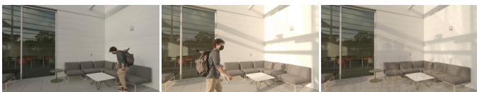
Fig. 12. From top to bottom, we show frame 0, frame 966 (last frame) and the extracted background. Since the lighting changes drastically during this scene, the extracted background contains a lot of ghosting artifacts.
