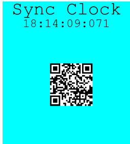
Figure 2. Digital clock and the randomly moving QR code pattern used to perform synchronization. We have two ways to do synchronization: (1) matching the timestamp; (2) aligning the QR code location in all views. We use these methods to ensure the synchronization is accurate enough.
