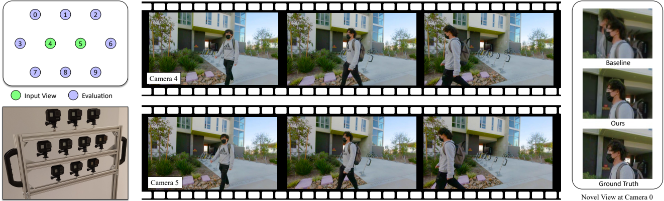
Figure 1. Our custom camera rig. Top left figure shows the configuration we use for evaluation in Sec. 5. We show the input stereo image sequences from camera 4 and camera 5 in the middle. Rightmost column shows the crops of rendered novel view at camera 0. Artifacts appear when the novel view is translated by a larger distance. We use conventional MPI method [28] as our baseline algorithm. Note how the area on top of the person’s head is distorted and shows “stack of cards” artifacts. This type of artifact flickers in a dynamic video as the network hallucinates the disocclusion per-frame.
