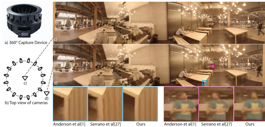
Fig. 1. We use 360° image data captured from a Yi-Halo camera (a), which consists of a ring of cameras as shown in (b). We present a learning based approach to reconstruct novel Multi Depth Panoramas (MDP) from these multi-view images, which can synthesize novel view images with both rotational and translational motions. We show panorama results using our MDPs from the center of the device (c) like the standard panorama synthesis, and also from a translated position (d) out of the rig. Note how the camera moves toward the counter. Our method accurately reproduces challenging disocclusion effects as shown in the cropped insets, which are significantly better than previous state-of-the-art methods that are based on RGBD representations [1, 27]. For better details on all the figures, please view the electronic version of this paper.
