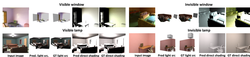
Fig. 9. Light source prediction on our synthetic dataset for four types of light sources. We visualize light source geometry and direct shading E_j without occlusion. Our method recovers both geometry and radiance of four types of light sources reasonably well.
