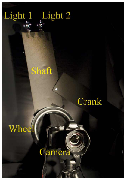
Fig. 17. A simple acquisition setup that exploits the fact that our approach does not require calibrated light source positions.
