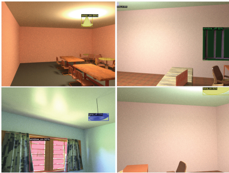
Fig. 28. Light source detection and instance segmentation results on the OpenRooms dataset [29].
