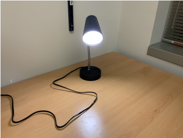
Fig. 30. A example where an indoor lamp is not symmetric and does not emit light uniformly in every direction.
