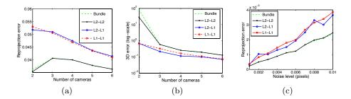
**Fig. 3.** (a) and (b) show reprojection and 3D errors, respectively, for triangulation with one outlier. Despite a higher reprojection error, the  $L_1$ -algorithms better bundle adjustment in terms of 3D error. (c) Reprojection errors for camera resectioning.
