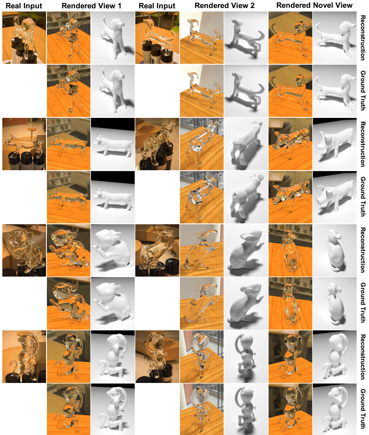
Figure 14. Results on 3D reconstruction for four real transparent objects. All shapes are reconstructed from 10 views, except the monkey in the last row that uses 12 views. We first present reconstruction results from two input views (columns 1-6). From left to right, the odd rows show the input image and the reconstructed shapes under different lighting and materials. The corresponding outputs using the ground-truth shapes rendered from the same view are shown in the even rows. We also render the reconstructed shapes and ground-truth shapes from a novel view direction that has not been used to build the visual hull (columns 7-8). In each instance, we observe that the reconstructions are close to the ground truth despite the challenging shapes, complex light paths and small number of views used for 3D reconstruction.
