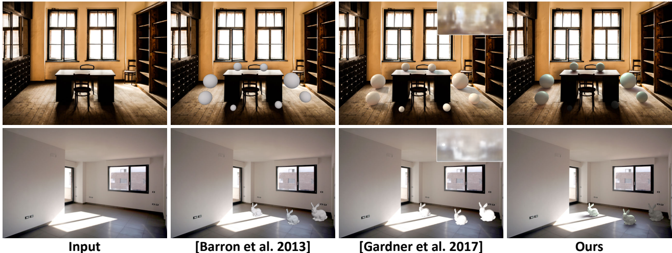
Figure 2. Comparison of object insertion results on a real image. Barron et al. [6] predict spatially varying log shading from a RGBD image, but their lighting representation does not preserve high frequency signal and cannot be used to render shadows and inter-reflections. Gardner et al. [20] predict a single lighting for the whole scene and therefore cannot model spatially varying indoor lighting. In contrast, our method solves the indoor scene inverse rendering problem in a holistic way, which results in photorealistic object insertion. The quality of our output may be visualized in a video for the example at the top, generated without any temporal constraints, at this link .
