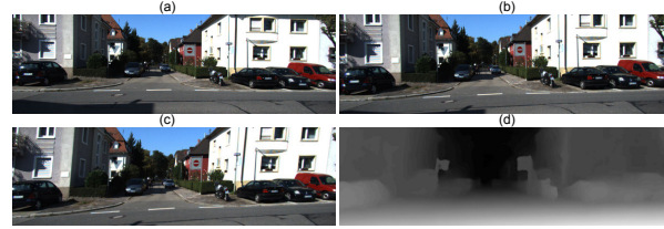
Figure 4. Example outputs at various steps in our training data synthesis: (a) original GS image, (b) GS image transformed by a homography, (c)(d) interpolated RS image and depth map.
