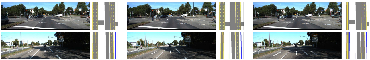
Figure 7: Qualitative results comparing H-BEV+DA and H-BEV+DA+GM in consecutive frames of two example sequences of the KITTI validation set. In each column, we have visualized the perspective RGB image, prediction from H-BEV+DA and that of H-BEV+DA+GM from left to right. Each row shows a sequence of three frames. We can observe more consistent predictions, e.g. , width of side-road and delimiter width, with the help of the temporal CRF.
