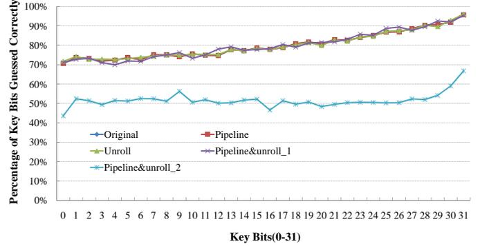
Fig. 5. The percentage of key bit guessed correctly for RSA architectures optimized for performance, i.e., those generated from high level synthesis from Table II.
