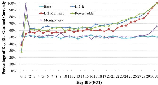
Fig. 7. Percentage of key bit guessed correctly for RSA architectures with mitigation techniques.
