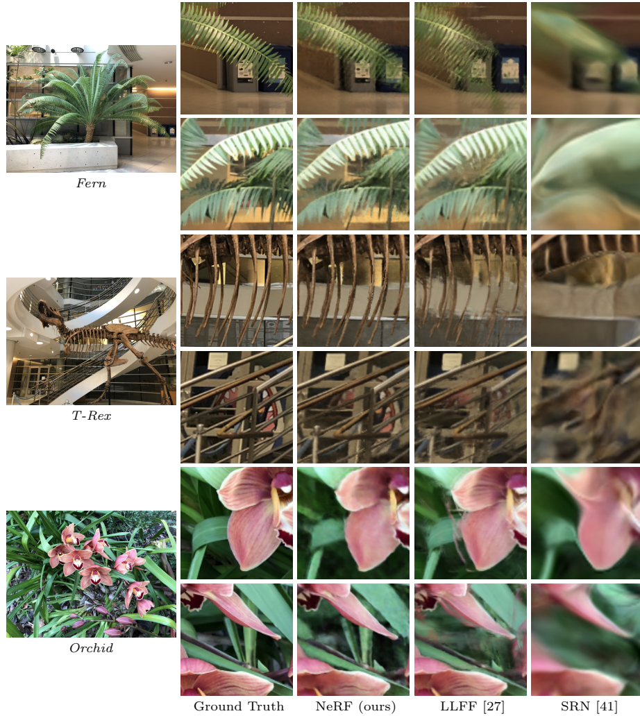
Fig. 6: Comparisons on test-set views of real world scenes. LLFF is specifically designed for this use case (forward-facing captures of real scenes). Our method is able to represent fine geometry more consistently across rendered views than LLFF, as shown in Fern ’s leaves and the skeleton ribs and railing in T-rex . Our method also correctly reconstructs partially occluded regions that LLFF struggles to render cleanly, such as the yellow shelves behind the leaves in the bottom Fern crop and green leaves in the background of the bottom Orchid crop. Blending between multiples renderings can also cause repeated edges in LLFF, as seen in the top Orchid crop. SRN captures the low-frequency geometry and color variation in each scene but is unable to reproduce any fine detail.
