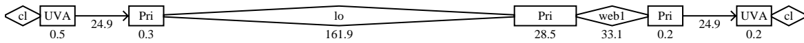
Figure 12: Linking algorithm output for a CoDeeN miss path with DNS lookup, delays in ms.
