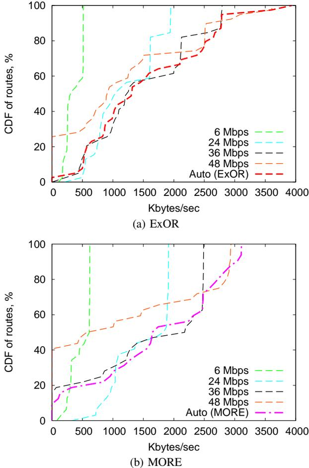
**Figure 5: Throughput of ExOR and MORE with automatic and various fixed rate selections. ALIX network with full power.**
