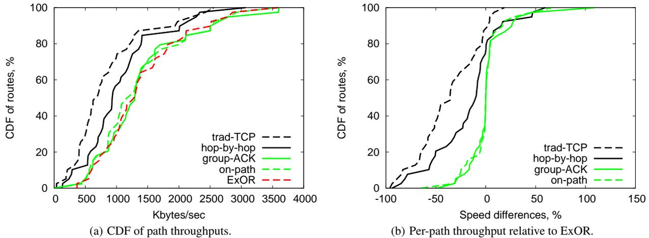
Figure 9: The performance of various flavors of the ExOR algorithm. ALIX network, power 30.
