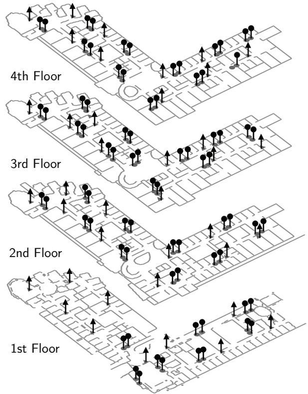
**Figure 1: The UC San Diego Jigsaw wireless testbed. We use the Jigsaw mesh nodes (depicted as circles); production 802.11 access in the building is provided by infrastructure-mode access points (shown as triangles).**
