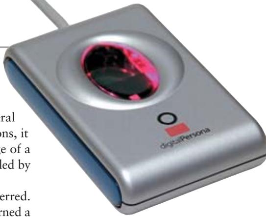
But because the device uses several LEDs shining in different directions, it obtains a three-dimensional image of a fingerprint and hence can't be fooled by a two-dimensional copy.
