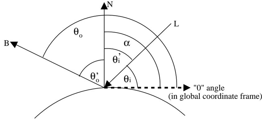
Figure 2. Diagram showing the geometry, with local and global coordinate angles marked. Note that angles are signed; in particular,  $\theta'_i$  is negative. The fact that  $\alpha$  is nearly a right angle has no significance and is only for convenience in illustration.
