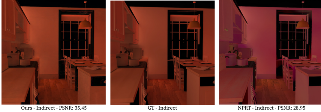
Figure 4: Comparison of our method with NPRT on DIFFUSE KITCHEN evaluated on a red environment map dissimilar to lighting conditions seen during training. In addition to an overall tone shift, the shading on certain objects (such as the pots on the stove) is inaccurate for NPRT, indicating our method is better able to generalize to unseen lighting conditions even for purely diffuse objects.
