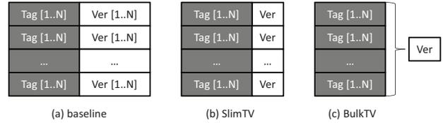
**Figure 3. Space Overhead of SlimTV and BulkTV.** Compared to the baseline where each tag requires version information, SlimTV uses a version information for a whole tag vector. BulkTV further reduces the space overhead by sharing a single version number across a range of memory addresses. Each row corresponds to the shadow memory information for a single address.
