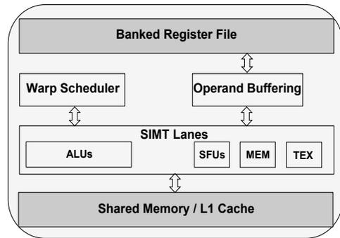
Fig. 3. Streaming Multiprocessor (SM) architecture.
