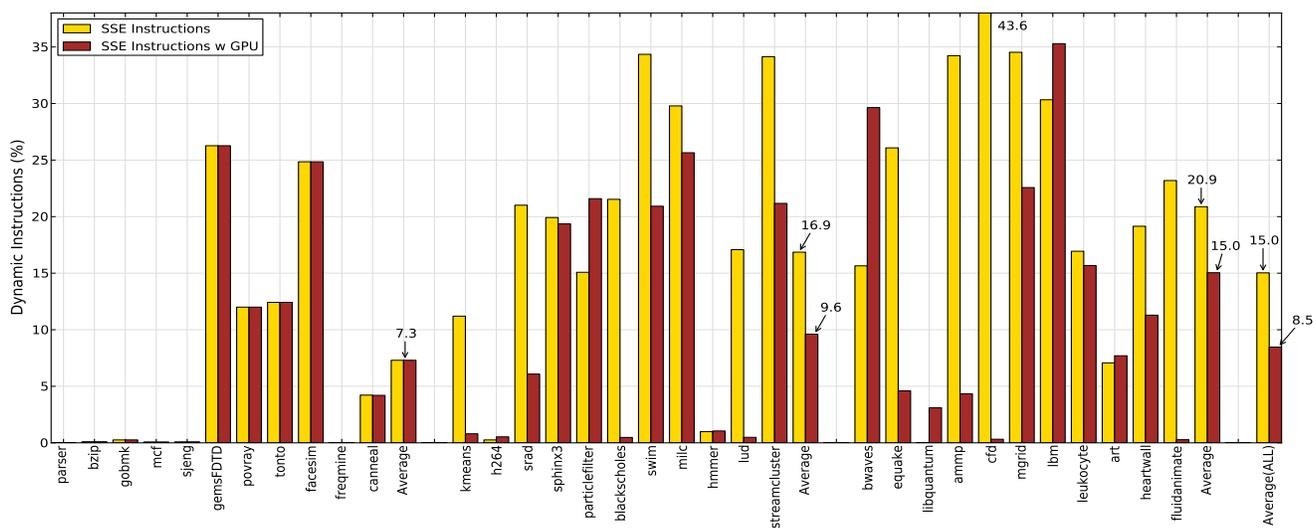
Fig. 13. Frequency of vector instructions with and without GPU.
