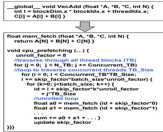
Fig. 18. GPU kernel and the generated pre-execution program.
