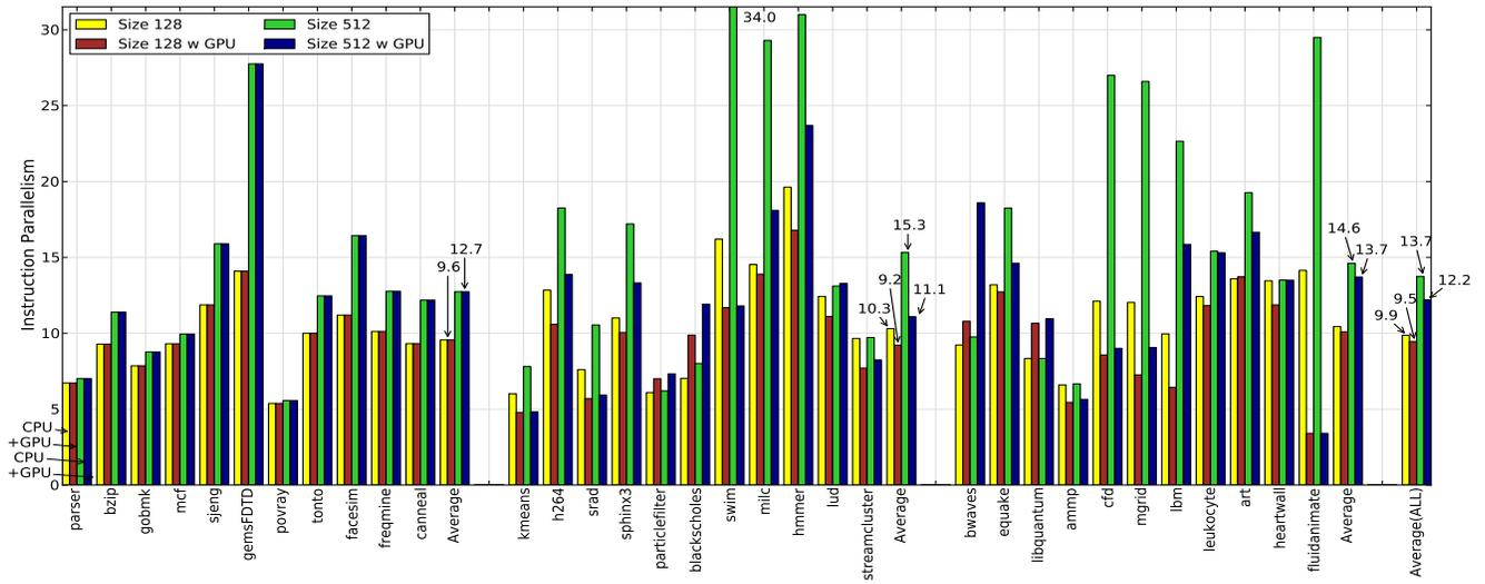
Fig. 10. Instruction level parallelism with and without GPU.
