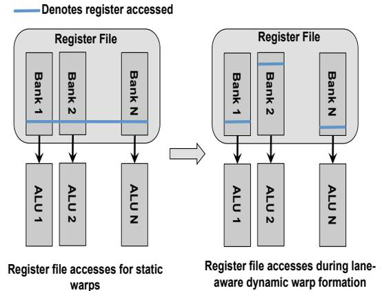
Fig. 7. Register file accesses during dynamic warp formation.
