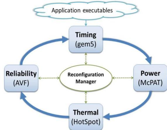
Figure 1: Proposed simulation methodology
