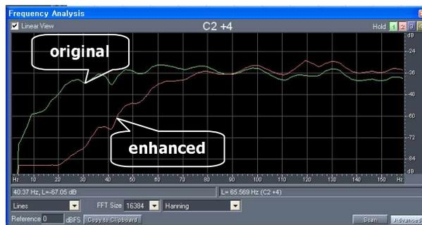
Figure 10 Bass level comparison of the original and the enhanced signals
