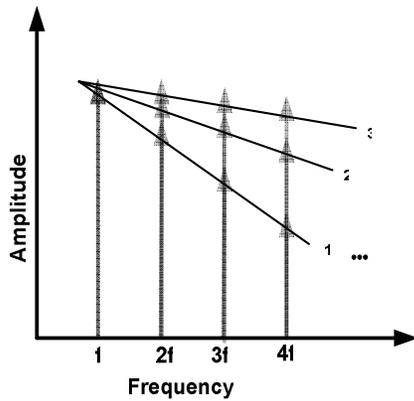
Figure 5: Harmonic spectrum envelope changes using 3 different fall time settings.
