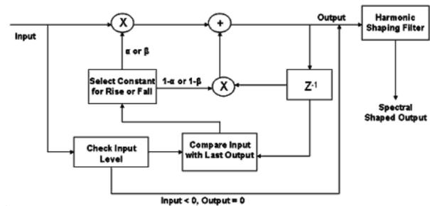
Figure 8: Harmonic generation method 2 block diagram.
