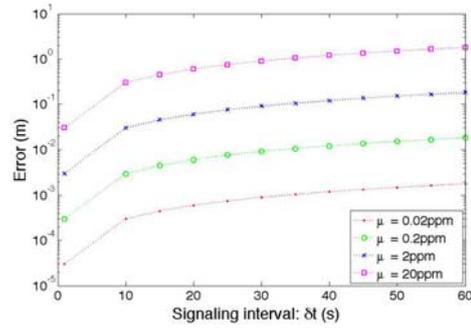
Figure 3: Error in distance due to the clock drift
