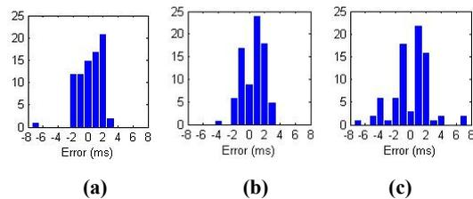
**Figure 13: Histogram of error in estimated clock offset using ToA-TS when speed is 0.8 m/s and signaling interval is (a) 10 s (b) 20 s, (c) 60 s**
