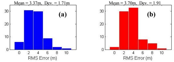
**Figure 9: Histogram of the RMS Error in position estimates for (a) ToA-TS and (b) TDoA for concurrent beacon signals**
