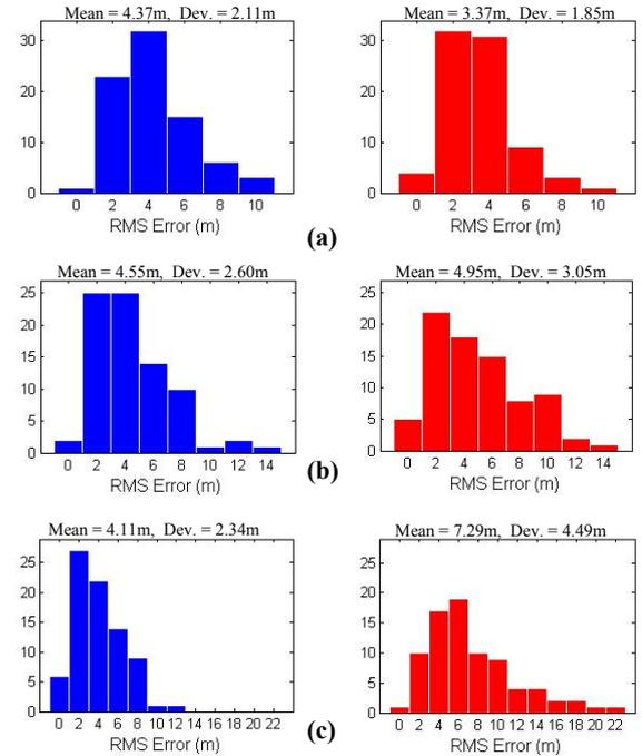
**Figure 10: RMS error in position estimates for ToA-TS (left) and TDoA (right), signaling interval 10 s and submersible's speed equal to (a) 0.2 m/s (b) 0.8 m/s (c) 1.6 m/s**
