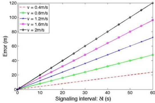
Figure 2: Error in distance due to the submersible's motion
