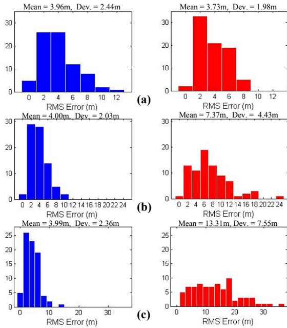
**Figure 11: RMS error in position estimates for ToA-TS (left) and TDoA (right), signaling interval 20 s and submersible's speed equal to (a) 0.2 m/s (b) 0.8 m/s (c) 1.6 m/s**
