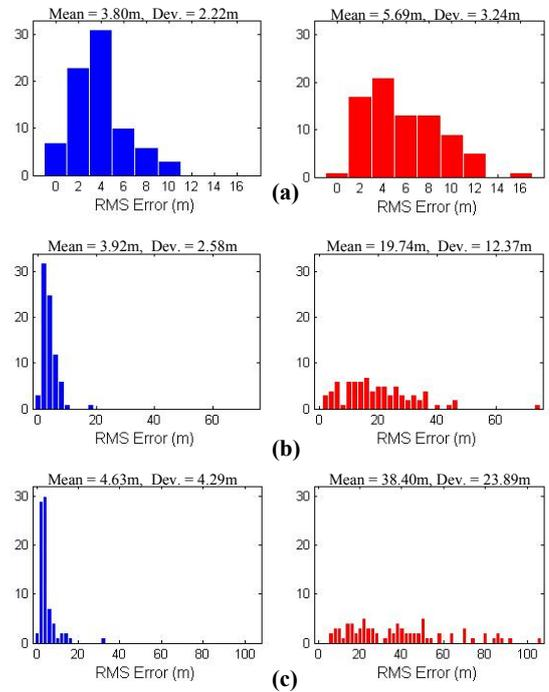
**Figure 12: RMS error in position estimates for ToA-TS (left) and TDoA (right), signaling interval 60 s and submersible's speed equal to (a) 0.2 m/s (b) 0.8 m/s (c) 1.6 m/s**
