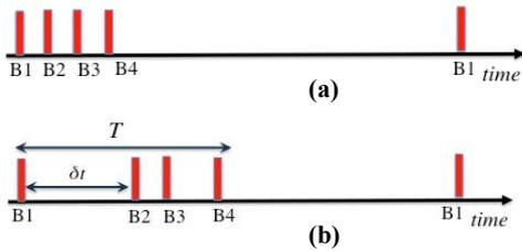
**Figure 1: Signals received at a submersible from four beacons in (a) LBL systems and (b) Swarm systems**
