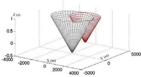
**Figure 8: Reduction in the uncertainty of position and clock offset by intersecting two independently computed cones in 3D**
