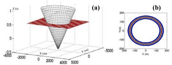
**Figure 7: (a) 3D pdf of position and clock offset given the measured time of flight of an acoustic message (b) Cross-section of the pdf in 2D for a fixed value of clock offset**
