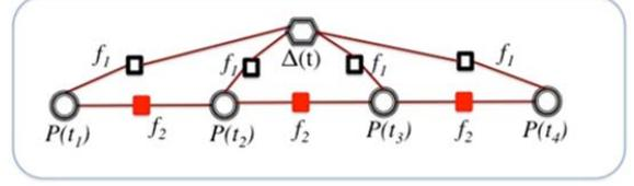
**Figure 4: Factor-graph description for joint synchronization and tracking**
