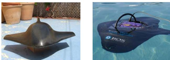
(a) Post carbon fiber fabrication. (b) Finished design with lid open.
