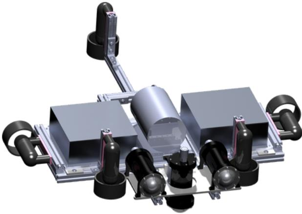
Fig. 14. A 3D drawing of the concept for Stingray 2.0. Shown are the chassis, five thrusters, two computer enclosures, a cylindrical battery enclosure on a small junction enclosure, and three camera enclosures.
