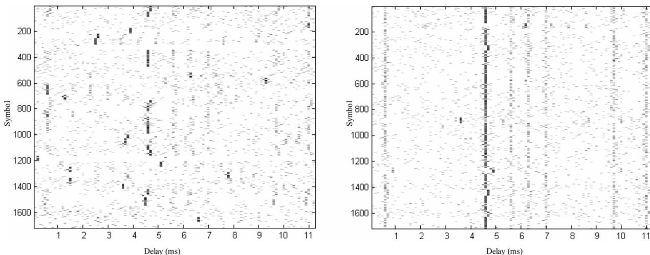
Figure 2. Estimated Multipath Intensity Profile (MIP) from simulations, actual number of multipaths = 10, SNR = -4 dB. Left: 2 training symbols, and estimated  $N_f$  varying from 1 to 16 with SER = 0.6645. Right: 5 training symbols, and estimated  $N_f$  varying from 5 to 16 with SER = 0.1023.
