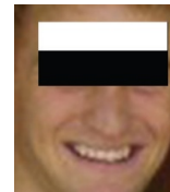
Figure 1. Example of a simple feature: a person's forehead is lighter than their eyes. This is an example of a 2 rectangle feature.
