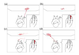
Figure 8: Dual-mode pointing. Ray-casting used for coarse-grained input (a). Activating precise mode via button press (b). Relative rotational movements control cursor movements (c). Switching back to coarse mode be releasing button (d). (Figure taken from [42].)
