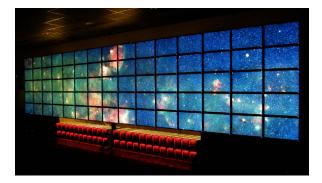
Figure 1: TACC's Stallion, the world's highest resolution display system weighing in at 328 megapixels [66].
