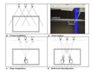
Figure 4: Touch detection via camera-based finger triangulation. (Figure taken from [61].)
