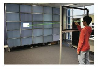
Figure 5: Using a transparent touch frame, users see the target on the distant display at their fingertips and perceive touching it directly. (Figure taken from [41].)
