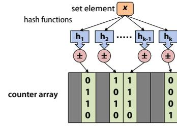
Fig. 3. A Counting Bloom Filter with 4-bit up/down counters.
