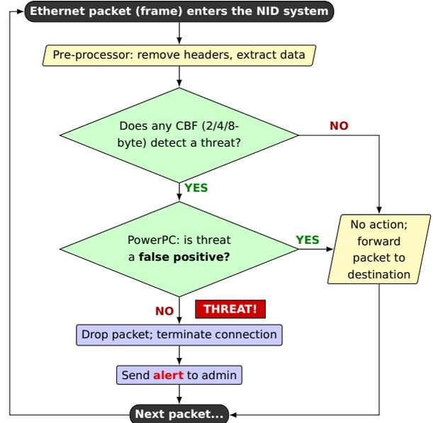
Fig. 7. Flowchart of Network Intrusion Detection using CBFs on an FPGA
