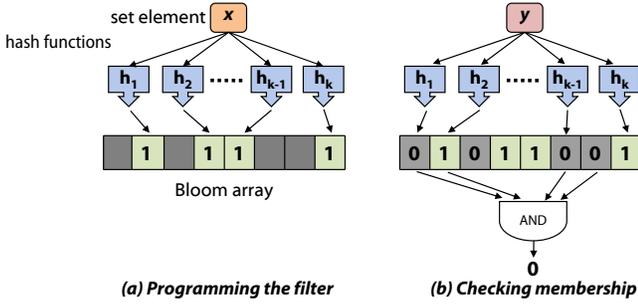
Fig. 2. (a) Programming a Bloom Filter (b) Querying a Bloom Filter; the data being checked is not a member of the set (AND=0)
