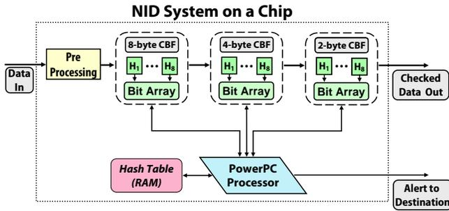
Fig. 5. A simplified block diagram of our NID design.
