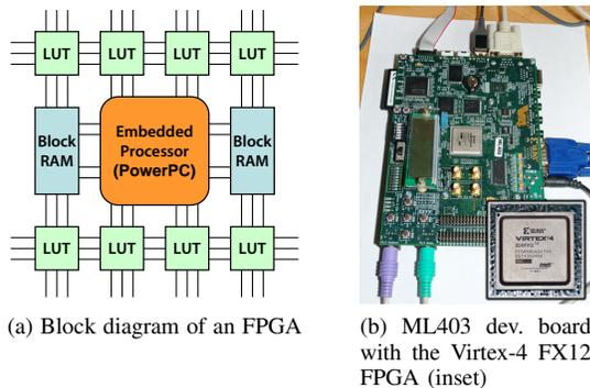
Fig. 4. FPGA structure and our FPGA system-on-chip
