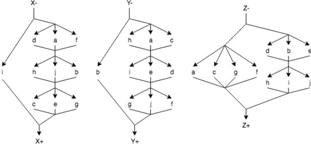
Fig. 5. Block partial order representation of the floorplan in Fig. 3.
