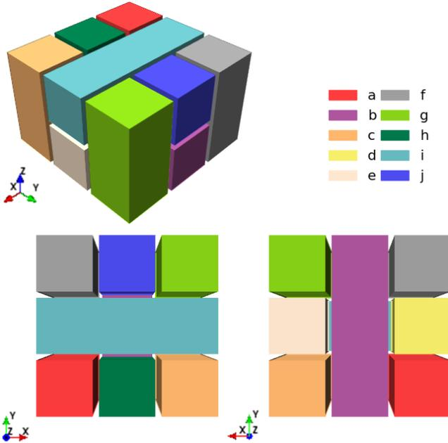
Fig. 3. A simple floorplan example. Top-left: isometric view. Top-right: block labels. Bottom-left: top (z-axis) view. Bottom-right: bottom (z-axis) view.
