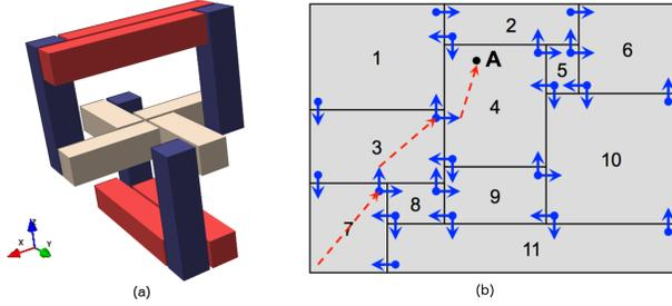
Fig. 2. Floorplan concept illustrations. (a) Nondegenerate neighbors - for the four gray blocks in the center, no block can shift against another due to the relative position of the red and blue outer blocks. (b) Corner-stitching - each blue arrow depicts stitch, which is pointer. Red dotted line shows the searching path for the block containing point A.
