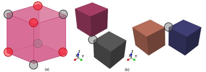
Fig. 8. Illustration of blocks corners for the purpose of the four trees representation: (a). red corners can have outgoing edges in the four trees representation to any neighboring corners in the floorplan, black corners do not have outgoing edges; (b). for any two neighboring black corners in a mosaic floorplan, there must be a red corner in the same neighborhood.
