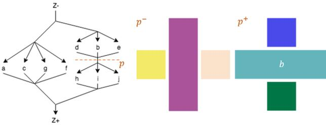
Fig. 6. A cutting plane in the example in Fig. 3. The two blueprints on the right are the footprints above and below the cutting plane  $p$ .
