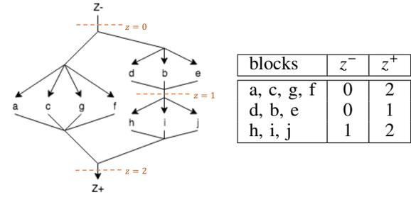
Fig. 10. Obtaining  $z$  dimension coordinates of all blocks from the  $z$  partial order of the example in Fig. 3.
