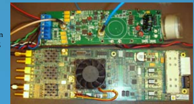
Fig. 5. Prototype hardware for one node. The hardware includes the transducer (ring in upper right corner), the analog circuit (upper board) and an DINI group's DNMEG_ADDA evaluation board. The two boards are connected via SMA cables.
