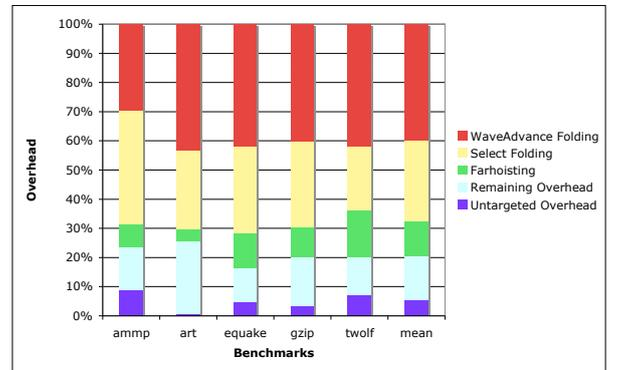
**Figure 12: The combined effect of eliminating instructions through WaveAdvance-Folding, Select-Folding, and Far-Hoisting on control instruction overhead. All sources of overhead, both eliminated and remaining, are a percentage of the original control overhead.**
