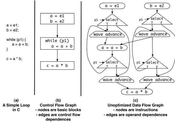
Figure 4: Example of a simple loop.
