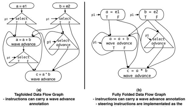
**Figure 11: Combining WaveAdvance-Folding and Select-Folding:** The dataflow graph for a simple loop that has been WaveAdvance-Folded (left) and then Select-Folded (right). The rightmost Select-Wave-Advance cannot be completely eliminated.
