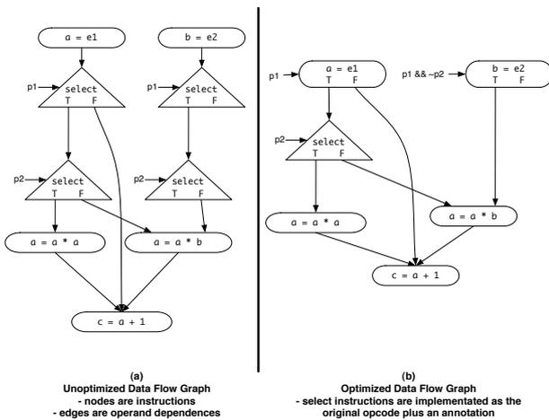
Figure 8: Select-Folding: The dataflow graph for an unoptimized nested branch (left) and with Select-Folding (right). For value ‘a,’ only one of the Select instructions folds, since folding the second would result in three destinations. For value ‘b,’ both Selects can be folded, since the predicates can be combined and the resulting instruction has only two destinations.
