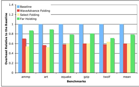
Figure 6: Instruction Overhead: The effect on control overhead of individually applying WaveAdvance-Folding, Select-Folding, and Far-Hoisting.
