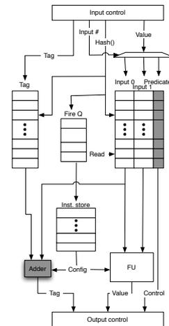
Figure 9: A WaveScalar Processing Element: The shaded elements – a third input queue and an adder – are added to each PE to enable WaveAdvance-Folding and Select-Folding, resulting in an increase in die area of only 2%.
