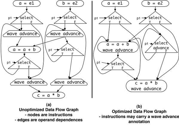
**Figure 5: WaveAdvance-Folding: The dataflow graph for an unoptimized simple loop (left) and with WaveAdvance-Folding (right).**
