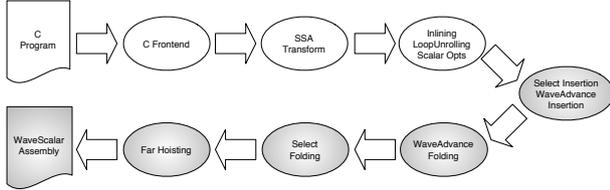
Figure 2: Compiler Flow: The WaveScalar compiler is based on the Scale compiler. Shaded boxes represent compilation passes added to compile and optimize WaveScalar code.
