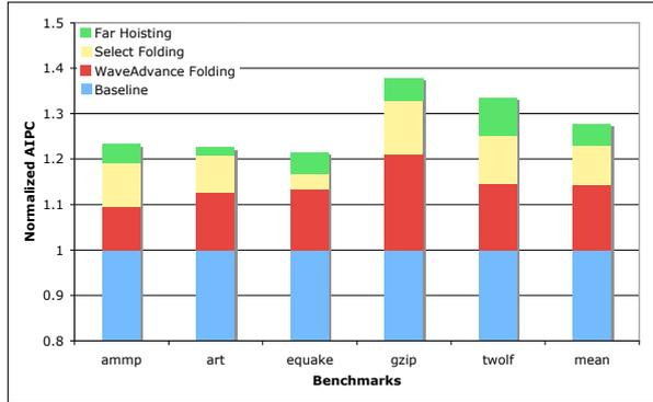
**Figure 13: The combined effect of WaveAdvance-Folding, Select-Folding, and Far-Hoisting on normalized AIPC.**
