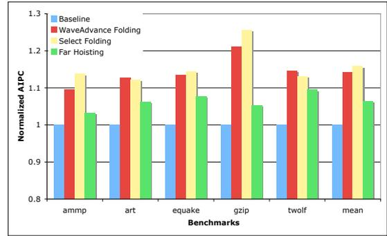
Figure 7: Performance: The effect on baseline performance of individually applying WaveAdvance-Folding, Select-Folding, and Far-Hoisting.
