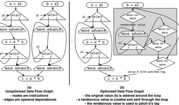
**Figure 10: Far-Hoisting:** The dataflow graph for an unoptimized loop (left) and with hoisting (right). In this example, a few extra instructions are required, but if enough values are hoisted out of the loop, the overhead required to patch the hoisted values' tags is more than offset by the reduction in Select and Wave-Advance instructions.
