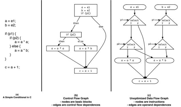
Figure 3: Example of branching code.
