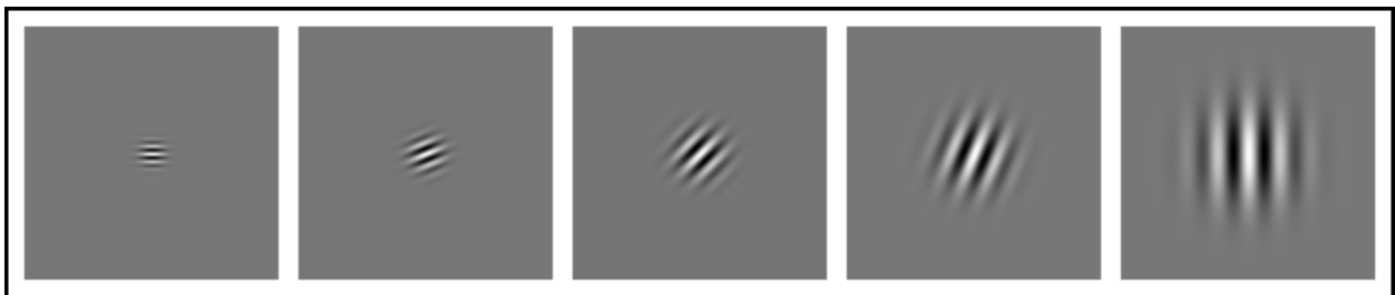
Figure 2: A set of Gabor filters of five different scales and orientations.
