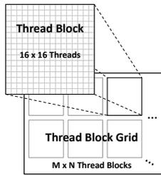
Figure 6. The grid consisting of thread blocks.
