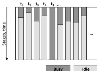
Figure 9. Running time of an imbalanced thread block.
