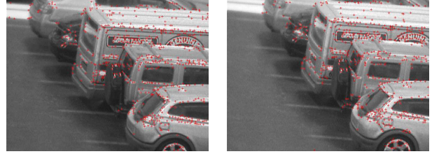
Figure 4: Harris corner detection results on a stereo pair of images.
