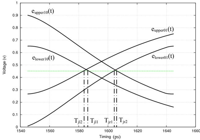
Figure 5. Timing jitter.
