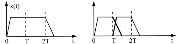
Figure 6. For signal with asymmetric rise/fall time, unit pulse response is not enough to cover all input patterns via superposition.
