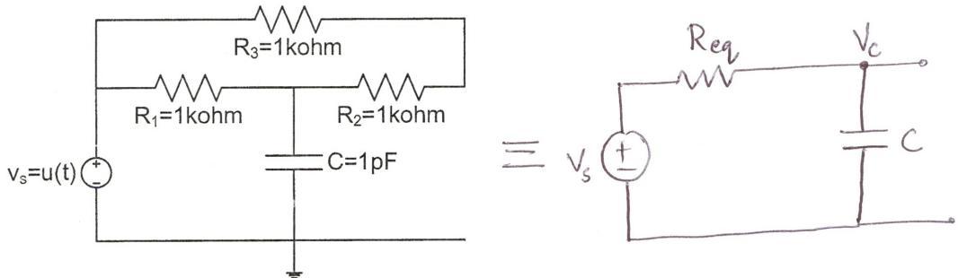
a. Derive the differential equation for the capacitor voltage,  $v_c(t)$ , given the initial condition that  $v_c(0) = 0\text{V}$ .
