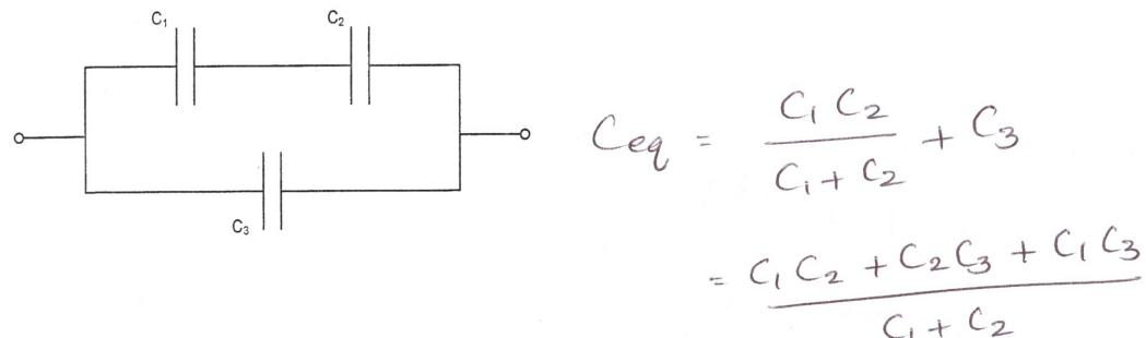
$$C_{eq} = \frac{C_1 C_2}{C_1 + C_2} + C_3$$
