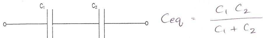
$$C_{eq} = \frac{C_1 C_2}{C_1 + C_2}$$
