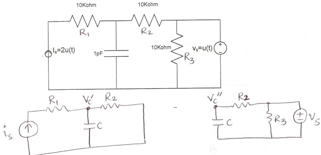
$$C \frac{dv'_c}{dt} + \frac{v'_c}{R_2} = i_s \rightarrow \textcircled{1} \quad C \frac{dv''_c}{dt} = \frac{v_s - v''_c}{R_2} \rightarrow \textcircled{2}$$
