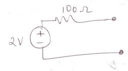
b. Derive the Norton's equivalent circuit of the network.
